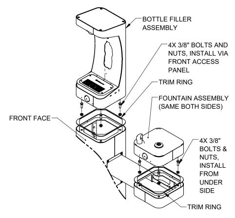
PLACE SQUARE TRIM RING ON BOTTOM OF BOTTLE FILLER AND PLACE BOTTLE FILLER ON TOP OF PEDESTAL, FACING THE FRONT. USE 3/8" BOLTS AND NUTS VIA THE FRONT ACCESS PANEL TO SECURE BOTTLE FILLER TO PEDESTAL. PLACE TRIM RING AND INSTALL FOUNTAINS ON ARMS AS SHOWN. CAREFULLY CENTER BOTTLE FILLER, FOUNTAIN, AND TRIM RINGS, THEN TORQUE BOLTS/NUTS TO 18 FT-LBS
