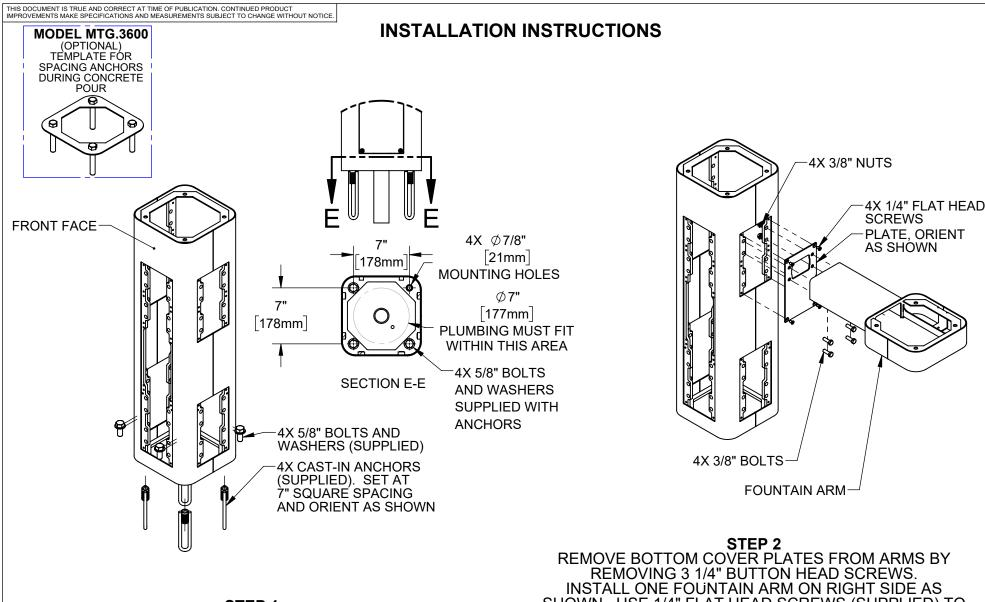
STEP 1 MOUNT PEDESTAL TO CONCRETE SLAB IN DESIRED ORIENTATION. SLAB TO BE 30" MINIMUM SQUARE AND 6" MINIMUM THICK (BY OTHERS). PLUMBING CAST IN CONCRETE MUST FIT IN 7" DIAMETER AREA CENTERED UNDER PEDESTAL LOCATION.
